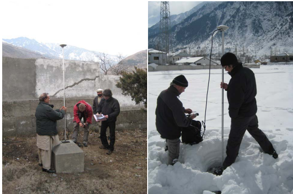
Figure 3.5: DGPS-Survey of SoP-Benchmarks in Swat Area at Madian (left) and Kalam in February 2008.
